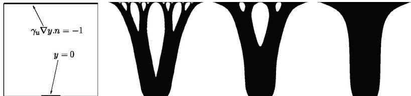
Optimal heater for \alpha = 0.1, 0.5, 2 , respectively (\gamma_1 = 1, \gamma_0 = 10^{-3}) .
